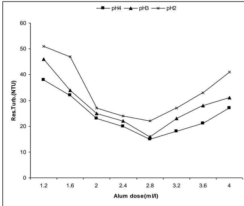
Fig.1b. Determination of optimum alum dose at 100NTU
