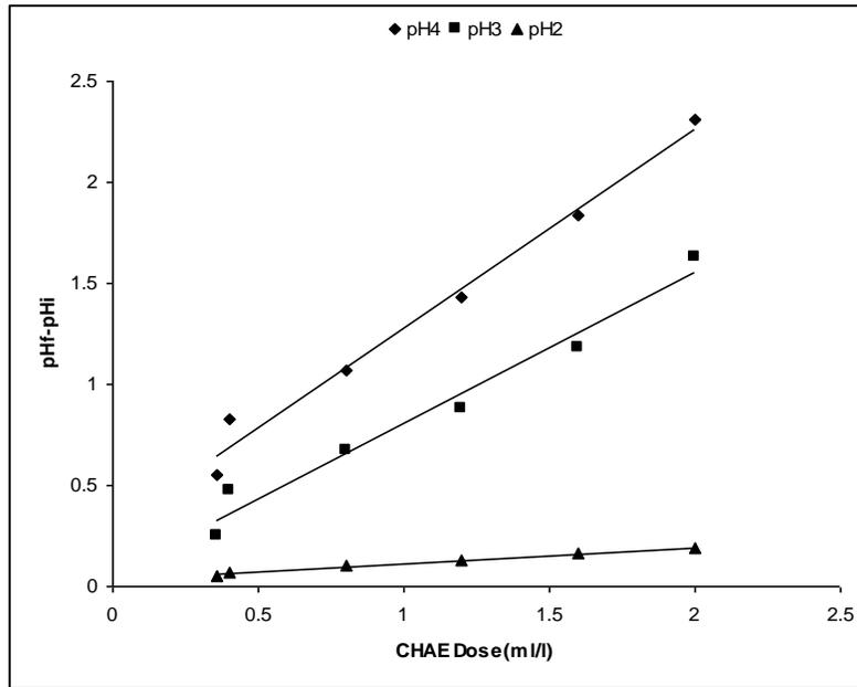
**Fig. 3b.** Linear correlation of  $\Delta\text{pH} = \text{pH}_f - \text{pH}_i$  versus CHAE dosage
