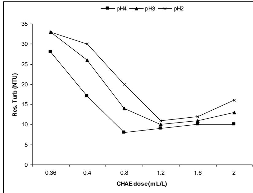
**Fig. 2c.** Effect of CHAE as coagulant aid at 50NTU (alum dose used = 1.0ml/L)
