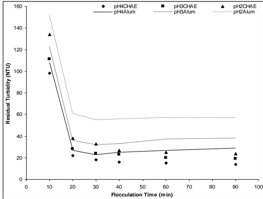
Fig. 4. Effect of flocculation time on residual turbidity at 300NTU
