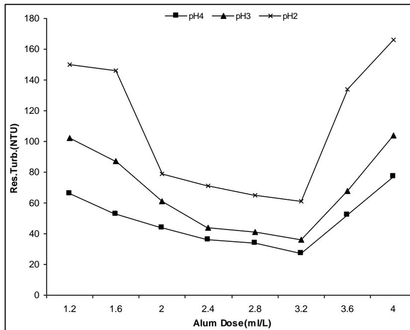
**Fig.1a.** Determination of optimum alum dose at 300NTU
