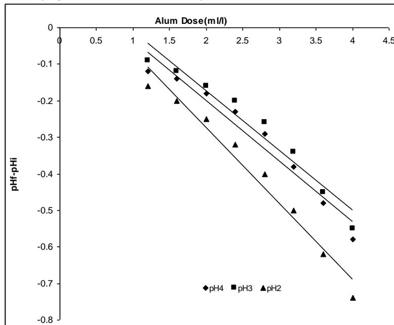
Fig. 3a. Linear correlation of  $\Delta\text{pH} = \text{pH}_f - \text{pH}_i$  versus alum dosage
