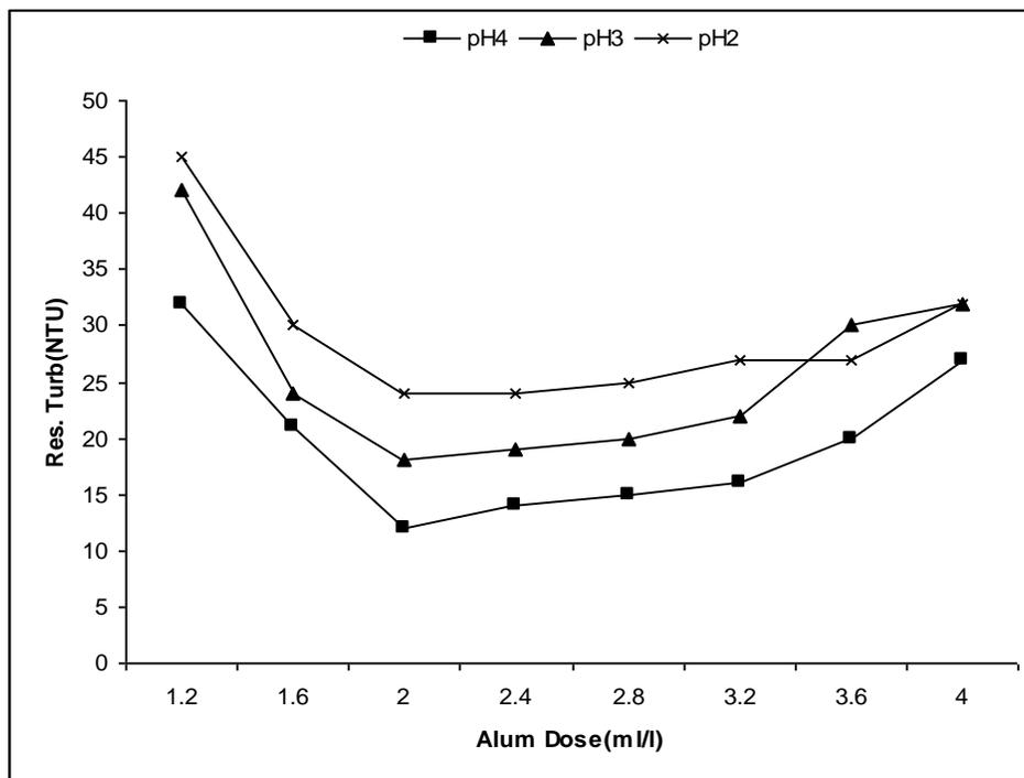
Fig.1c. Determination of optimum alum dose at 50NTU
