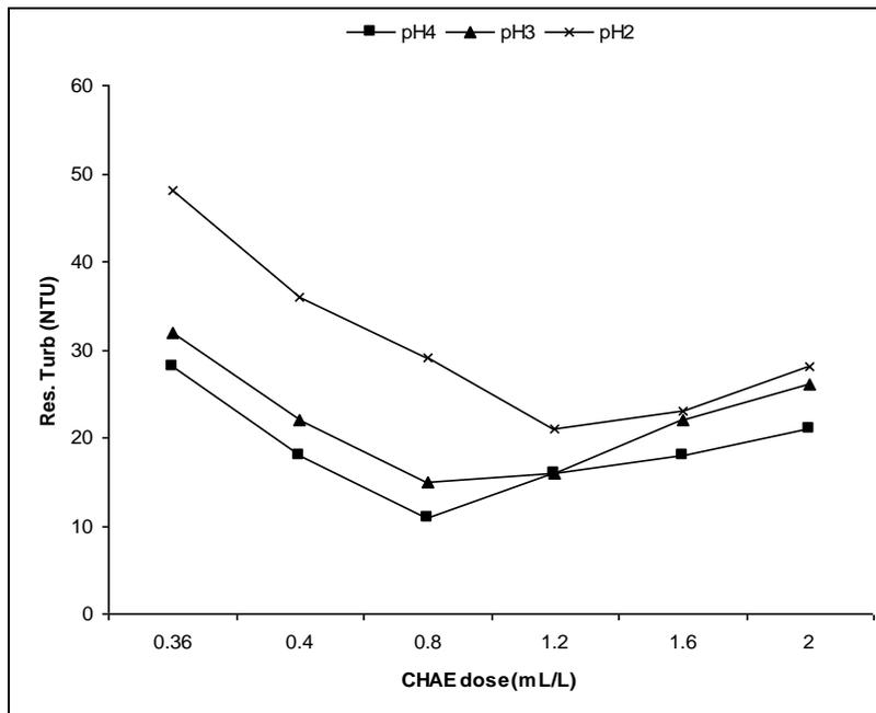
Fig. 2b. Effect of CHAE as coagulant aid at 100NTU (alum dose used = 1.4mL/L)
