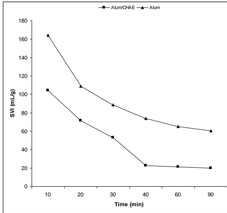
**Fig. 6.** Determination of sludge volume index
