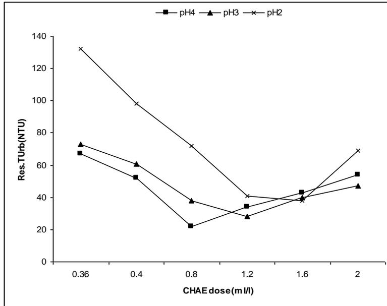
Fig. 2a. Effect of CHAE as coagulant aid at 300NTU (alum dose used = 1.6mL/L)
