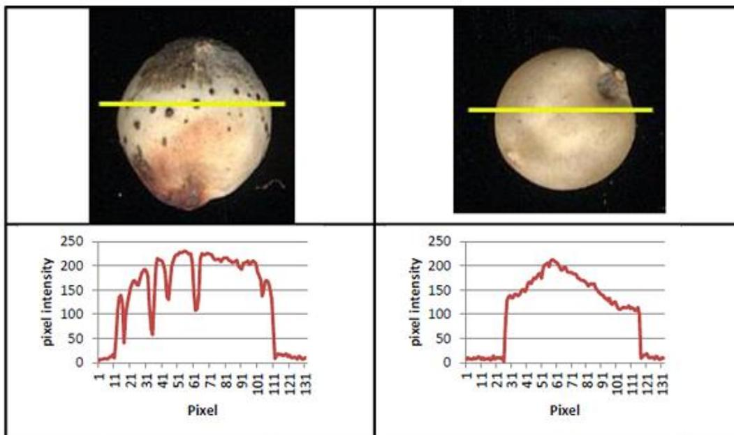
**Fig 3.** The spot identification algorithms use pixel intensity profile plots. Shown are example images and plots of fungal-infected (left) and non-infested (right) sorghum grains. Note how the dark spots on the infected grain cause the pixel intensity to drop sharply, whereas the non-infested grain profile plot is fairly smooth.
