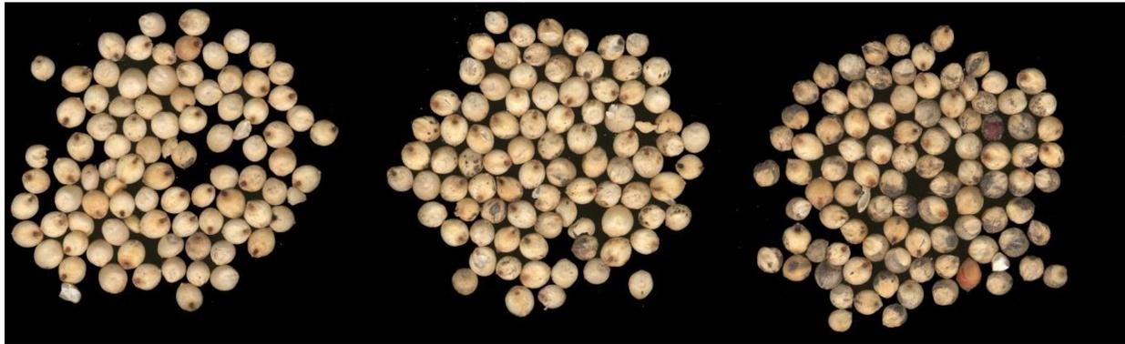
**Fig 4.** Images of each sorting fraction, (left) accept twice; (middle) accept once–reject once; (right) reject twice.
