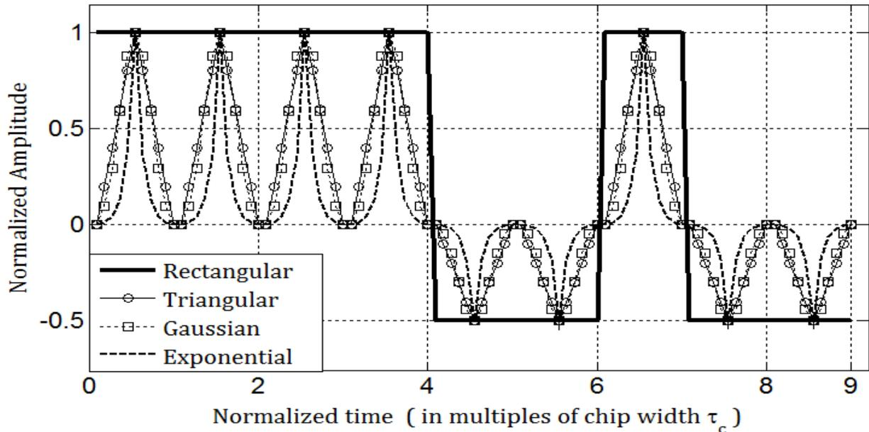
Fig. 3. Frank-9 phase coded pulse for rectangular, triangular, Gaussian, Exponential pulse shapes.
