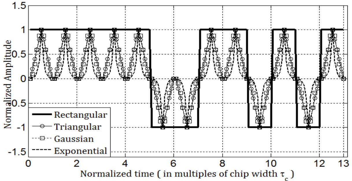
Fig. 2. Barker-13 phase coded pulse for rectangular, triangular, Gaussian, Exponential pulse shapes.
