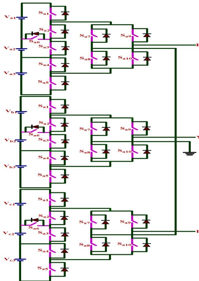
**Fig. 1.** Three Phase Seven Level Inverter
