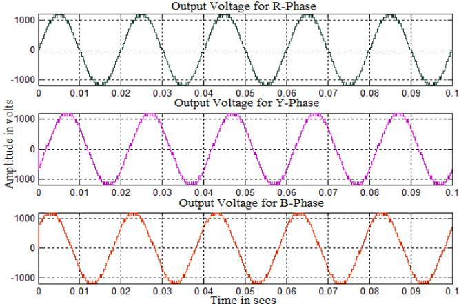
Fig. 7. Simulated output voltage generated by UAPODPWM technique for R-load
