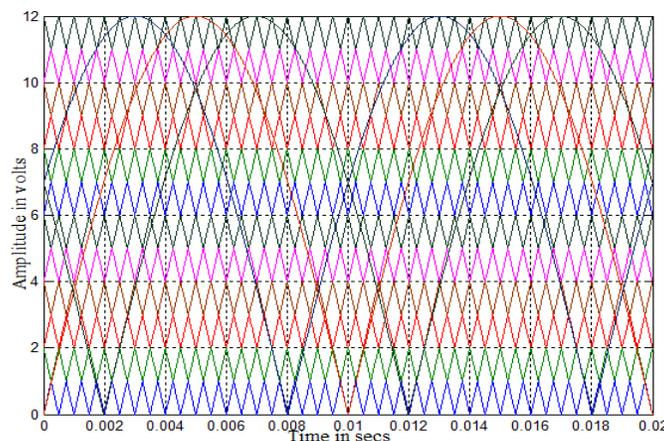
**Fig. 3.** Modulating and carrier waveforms for UAPODPWM strategy ( $m_a = 1$  and  $m_f = 40$  )
