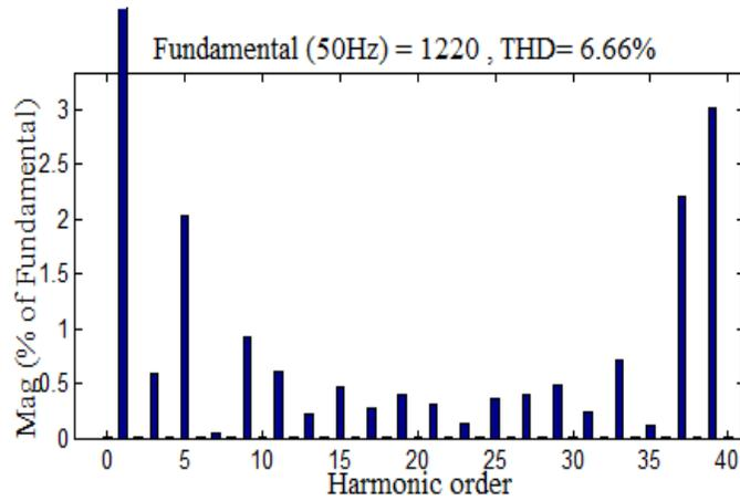
Fig. 13. FFT spectrum for UCOPWM technique
