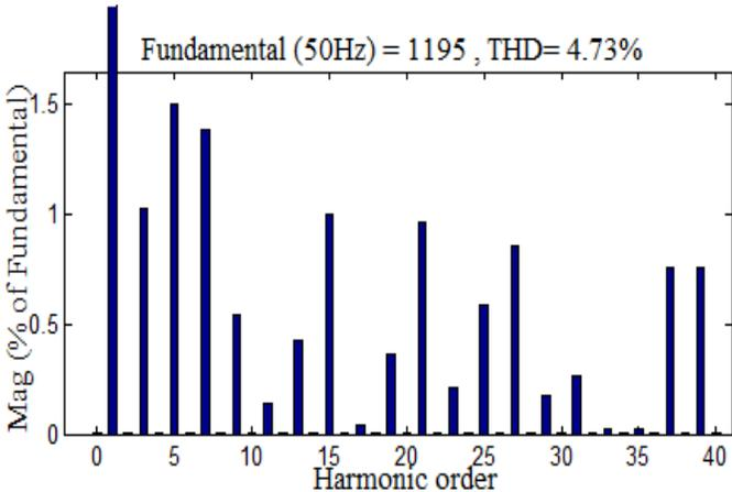
Fig. 11. FFT spectrum for UAPODPWM technique
