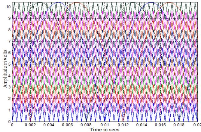
**Fig. 5.** Modulating and carrier waveforms for UCOPWM strategy ( $m_a = 1$  and  $m_f = 40$ )
