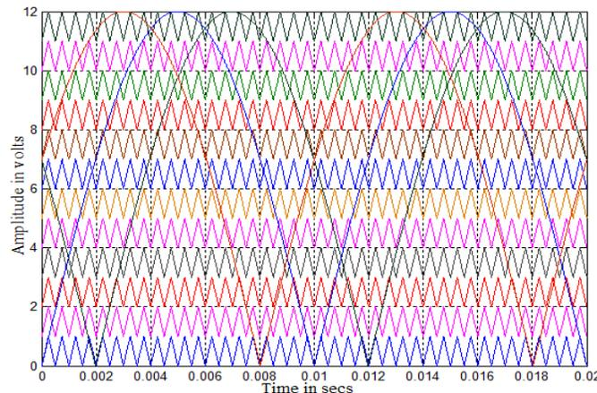
**Fig. 2.** Modulating and carrier waveforms for UPDPWM strategy ( $m_a = 1$  and  $m_f = 40$  )
