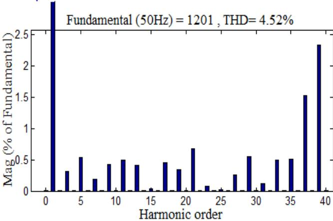
Fig. 10. FFT spectrum for UPDPWM technique
