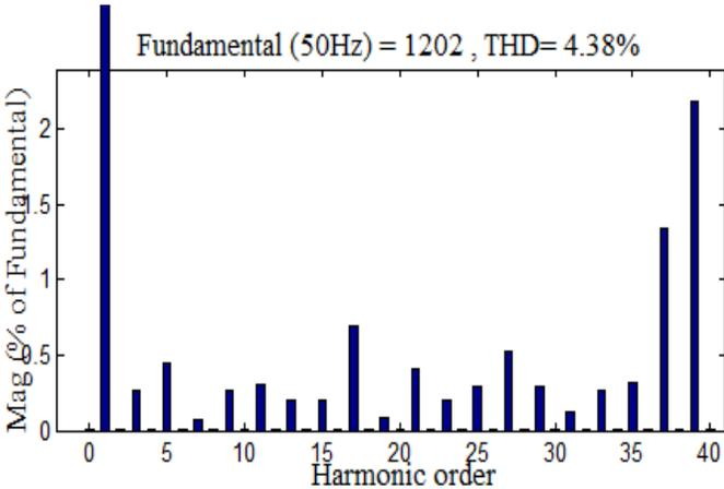
Fig. 12. FFT spectrum for UVFPWM technique
