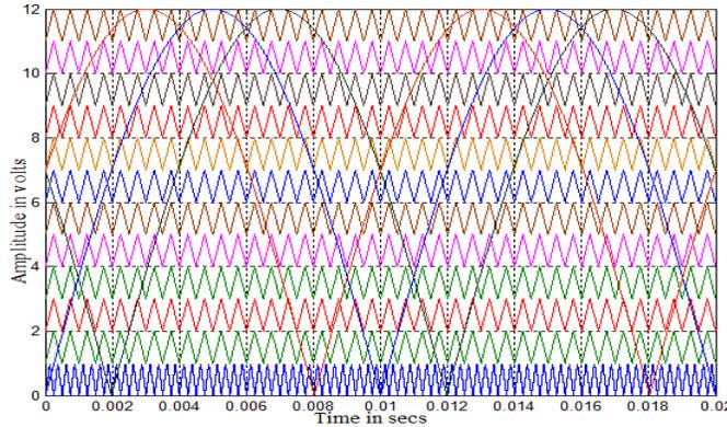
**Fig. 4.** Modulating and carrier waveforms for UVFPWM strategy ( $m_a = 1$  and  $m_f = 40$  for upper switches and  $m_a = 1$  and  $m_f = 80$  for intermediate switches)
