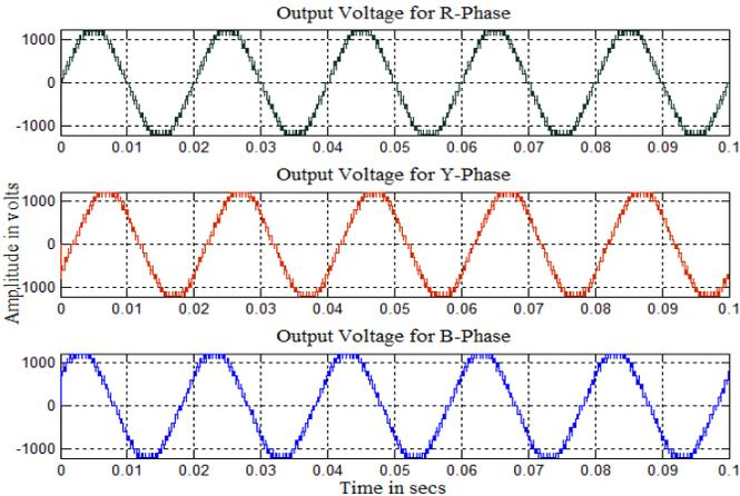
Fig. 9. Simulated output voltage generated by UCOPWM technique for R-load
