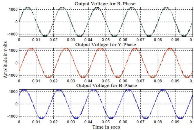
Fig. 6. Simulated output voltage generated by UPDPWM technique for R-load
