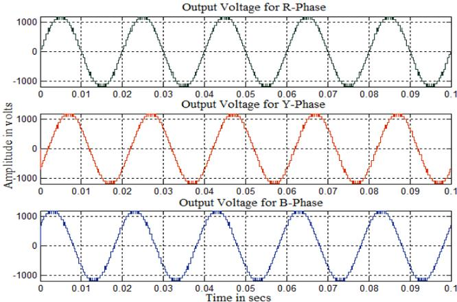
Fig. 8. Simulated output voltage generated by UVFPWM technique for R-load
