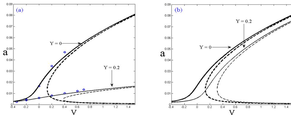
**Figure 4.** (a) Effect of IPD on the galloping vs.  $V$ ;  $u_1 = 0.1, \sigma = 0, \nu = 10$ , (b) effect of external excitation for the same values of parameters. (picked from Belhaq et al, 2013a; Mokni et al, 2014); Solid line: stable; dashed line: unstable; circle: numerical simulation.
