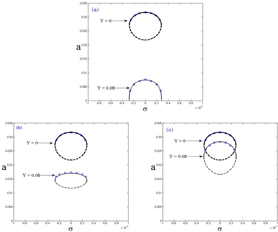
**Figure 9.** (a) Effect of  $Y$  of the FHE and the IPD on galloping, (b) effect of IPD on galloping vs.  $V$ , (c) effect of external excitation (picked from Belhaq et al, 2013a; Mokni et al, 2014),  $u_2 = 0.1$ ,  $V = 0.167$ ,  $\nu = 8$ . Solid line: stable; dashed line: unstable; circle: numerical simulation.
