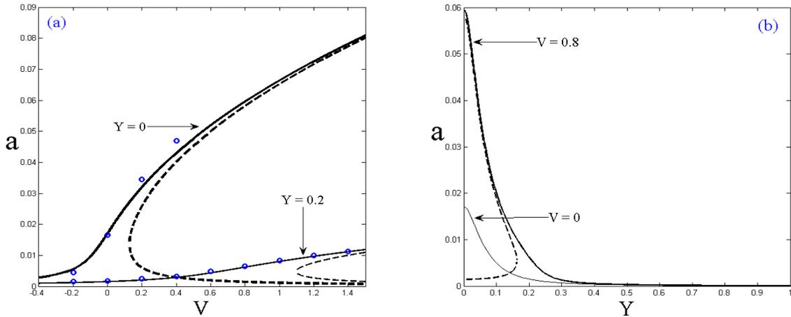
**Figure 3.** (a) Effect of combined FHE and IPD on the galloping amplitude vs.  $V$ , (b) variation of galloping vs.  $Y$ ,  $u_1 = 0.1, \sigma = 0, \nu = 10$ . Solid line: stable; dashed line: unstable; circle: numerical simulation.
