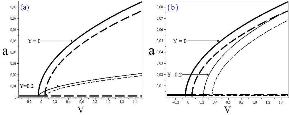
**Figure 8.** (a) Effect of IPD on galloping vs.  $V$ , (b) effect of external excitation (picked from Belhaq et al, 2013a; Mokni et al, 2014). Solid line: stable; dashed line: unstable; circle: numerical simulation;  $u_2 = 0.1, \sigma = 0, \nu = 8$ .
