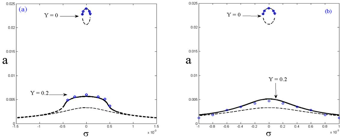
**Figure 6.** (a) Effect of the IPD on the galloping vs.  $\sigma$ , (b) effect of external excitation (picked from Belhaq et al, 2013a; Mokni et al, 2014). Solid line: stable; dashed line: unstable; circle: numerical simulation;  $u_1 = 0.033, \nu = 10, V = 0.117$ .
