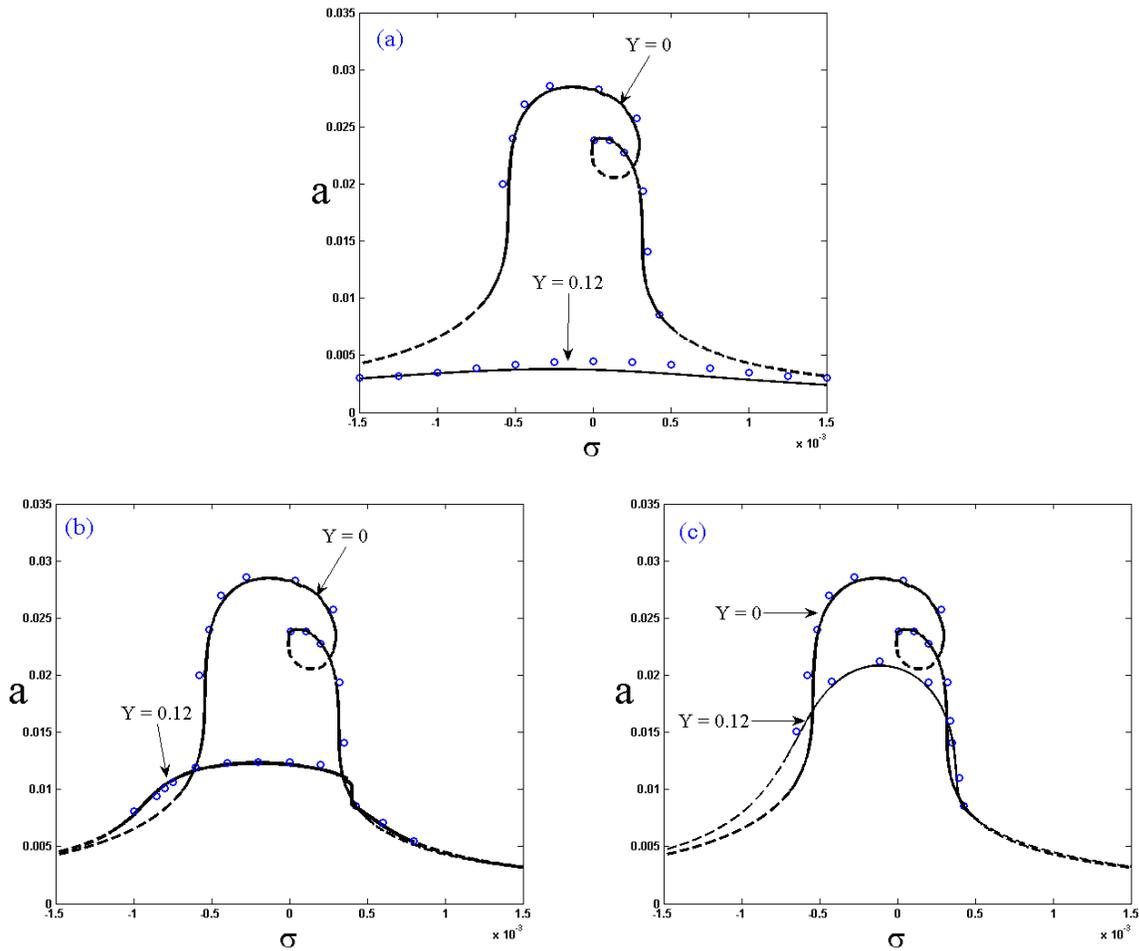
**Figure 10.** (a) Effect of  $Y$  of the FHE and the IPD on galloping, (b) effect of IPD and (c) effect of external excitation (picked from Belhaq et al, 2013a; Mokni et al, 2014) for  $V = 0.11$ ,  $u_1 = 0.1$ ,  $u_2 = 0.1$ . Solid line: stable, dashed line: unstable, circle: numerical simulation.
