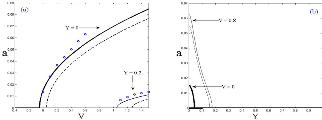
**Figure 7.** (a) Effect of  $Y$  on galloping;  $u_2 = 0.1$ ,  $\sigma = 0$ ,  $\nu = 8$ , (b) variation of galloping vs.  $Y$ . Solid line: stable; dashed line: unstable; circle: numerical simulation.
