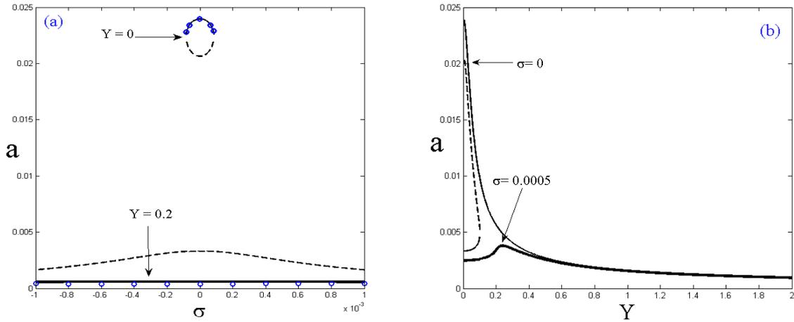
**Figure 5.** (a) Effect of FHE and IPD on the galloping amplitude vs.  $V$ , (b) variation of galloping vs.  $Y$ ,  $u_1 = 0.1, \sigma = 0, \nu = 10$ . Solid line: stable; dashed line: unstable; circle: numerical simulation.
